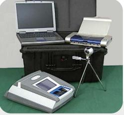
**Child Identification Solution** includes fingerprint scanner, digital camera, laptop, color printer and carrying case
